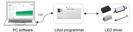
All the LED drivers that support Lifud programmer in our company can use LF-SCS080C programmer. Because of different product types, the wiring connecting the Lifud programmer to the LED driver will be different. Please follow the wiring instructions as specified in the product specification.
